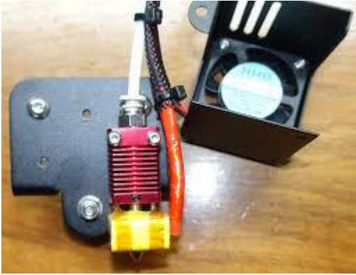
Stock Ender 3 hot end with insulation and Kapton tape wrap.
