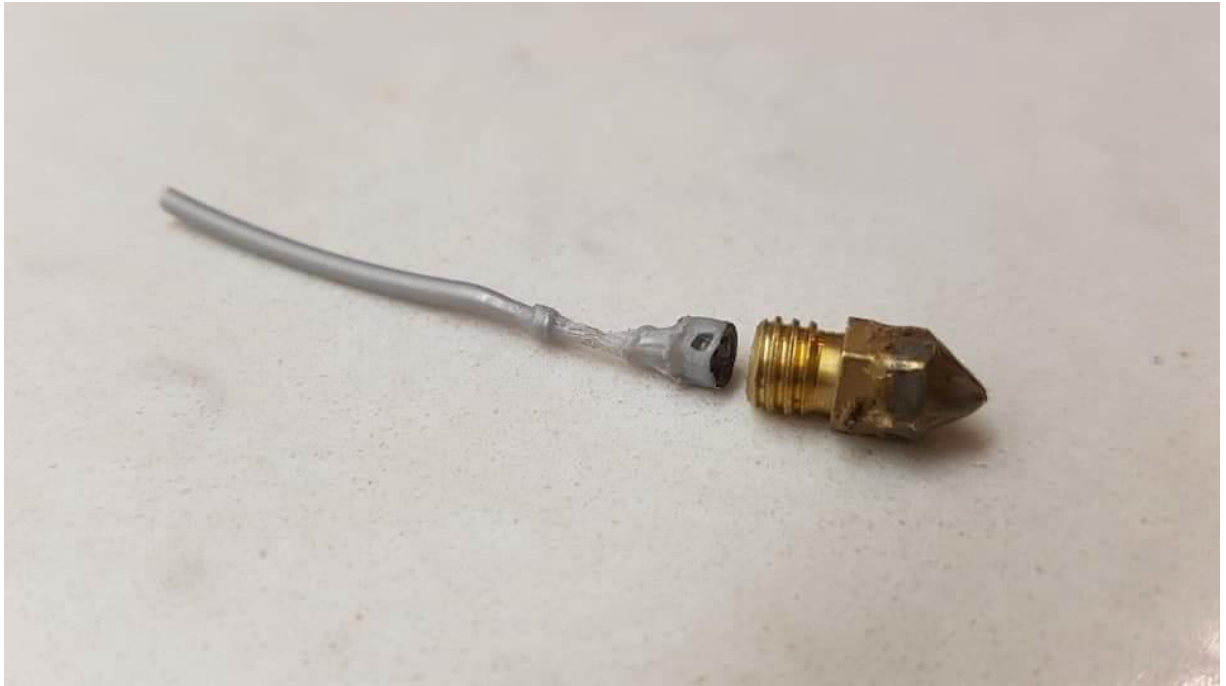
Figure 1 The PTFE pulled away about 2.5mm from nozzle in this discovery picture.
